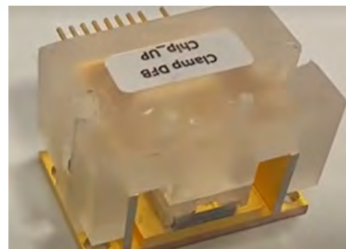
HHL package prototype developed for the QCL in the mid-IR sensor module.
